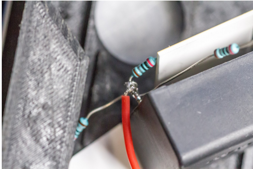
Figure 12: High-Voltage Supply Line on capacitor Anode
