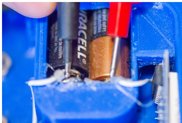
Figure 24: Input (battery) voltage measurement
